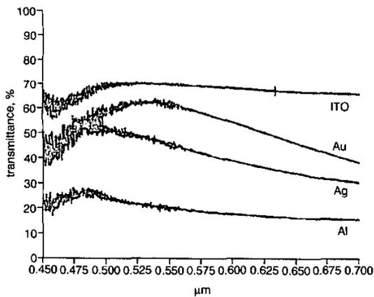
Fig. 3 Transmittances of metallic films compared to ITO in visible wavelength
